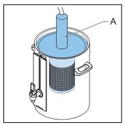
The tea filling pipe and filter unit (A) receive the hot water and combine it with a pre-loaded tea product inside the container.
