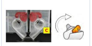
Clean the interior of the machine with a damp cloth. Remove any excess ingredients from the machine components and wash under warm water and dry thoroughly. Mount all the cleaned components to the original positions ENSURE all canisters are located back properly otherwise the product will not flow LEAVE mixing bowls damp to ensure seals do not split on mixer motor
